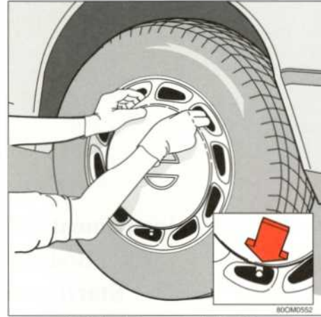
Pull the hubcap straight off
